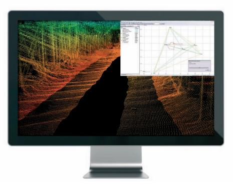
The POSPC module in POSPac MMS is used to combine the raw Lidar range measurements with the navigation data to generate point cloud data as above..
